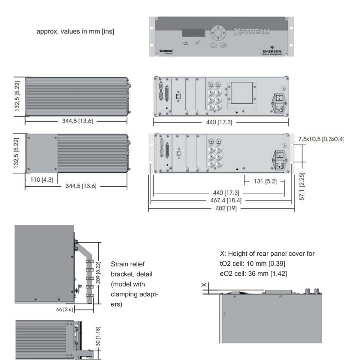
Fig. 2-5: X-STREAM X2GP - Dimensions
